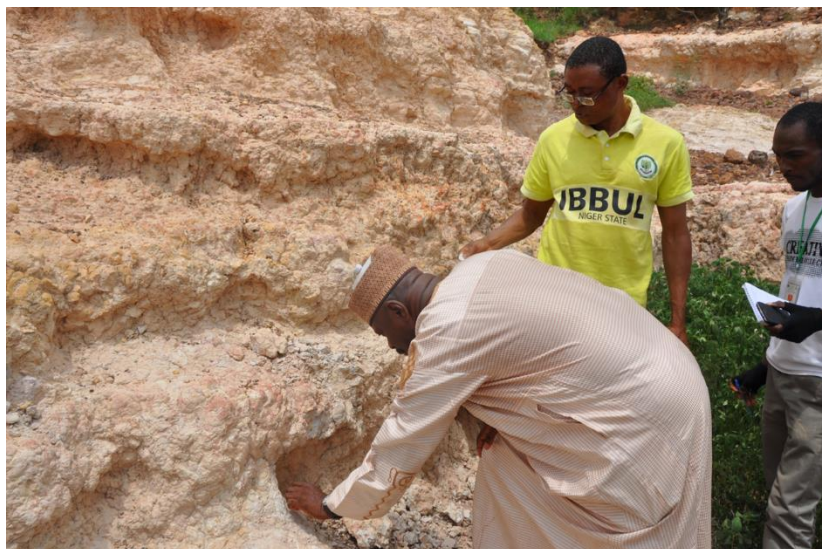
Fig. 5. Conducting textural examination on the clay deposit at Kutigi. Geochemical results show that this clay deposit (top-most layer 3) has the best quality (highest alumina and least silica content) amongst the clay deposits studied
